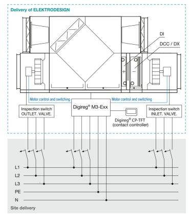
Note: Design of the main breaker and inlet cable to the Digireg<sup>®</sup> I/C system is part of electric project (the project is not within supply scope of ELEKTRODESIGN ventilátory, s.r.o.). Information on total electric ilet power of A/C unit is part of the unit technical specification.
