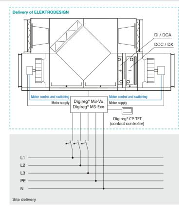
Note: Design of the main breaker and inlet cable to the Digireg<sup>®</sup> I/C system is part of electric project (the project is not within supply scope of ELEKTRODESIGN ventilátory, s.r.o.). Information on total electric inlet power of A/C unit is part of the unit technical specification.
