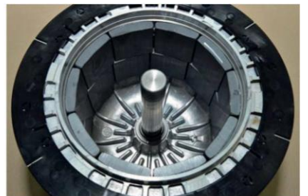
Rotor made of die-cast aluminium with plastic plate (not shown) on the ring
