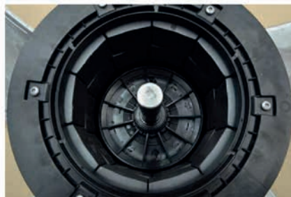
Steel rotor with plastic cooling wheel
