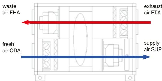
Arrangement diagram of components of Duovent® Compact RV units with mixing:
